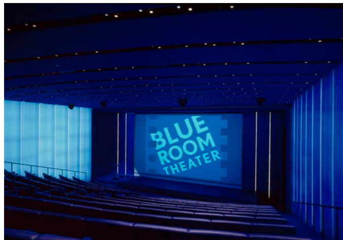
Looking north. Backlighting blue Polygal walls are at sides and LED lighted stripes are on each side of 32' screen.
