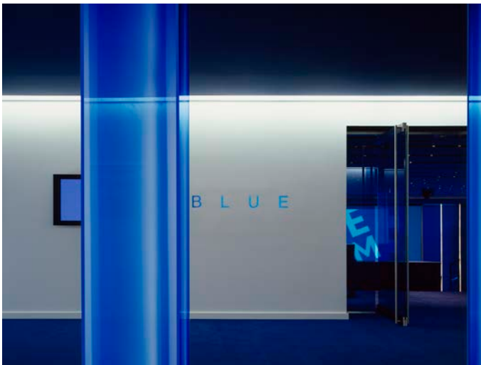
Fiber optic "BLUE" sign at entry with blue Polygal column covers backlighting by fiber optic lights.
