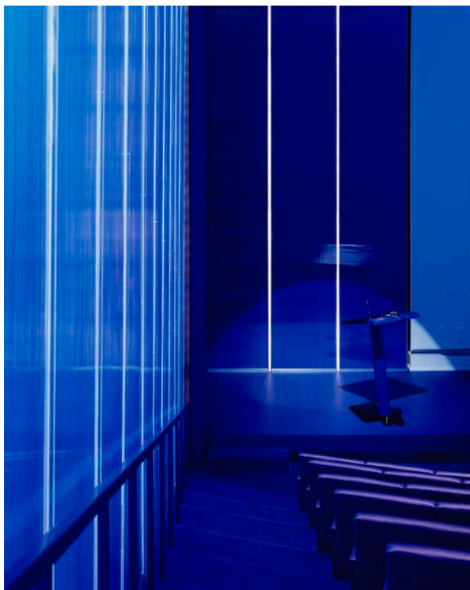
Blue podium is lit by motorized theatrical lights. Wall panels behind podium are blue Polygal that is front lit with white LED stripes.
