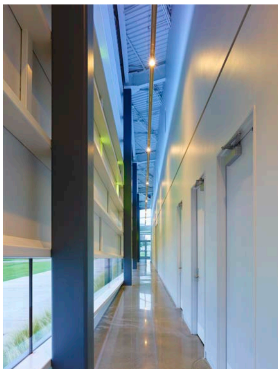
The west corridor looking north glows after sunset with the blue ceiling night light. The building shell is exposed with the exterior metal skin over a light steel frame. This solution is inspired by the rowing shell construction of fiberglass and aluminum.
