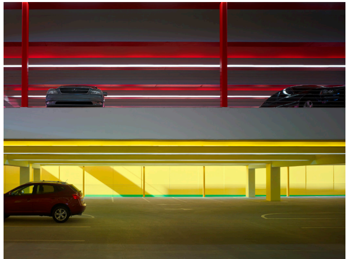
A view looking north as the entry ramp exposes the second level and the light illuminates the colored atrium edges. The lighting includes fluorescent down lighting and color uplighting for the individual levels.
