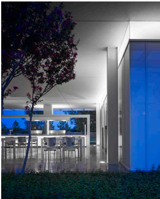
Dusk view looking west illustrating the lighting concept. LED ground lights, linear beam lighting, the counterface light and the clerestory windows combine to provide dramatic lighting.
