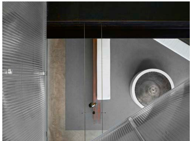
View from bridge looking down to seating on the ground level. Polycarbonate panel connections are visible as well as the cable lighting. The furniture includes a bench made from a steel beam and a table made from a concrete saw.
